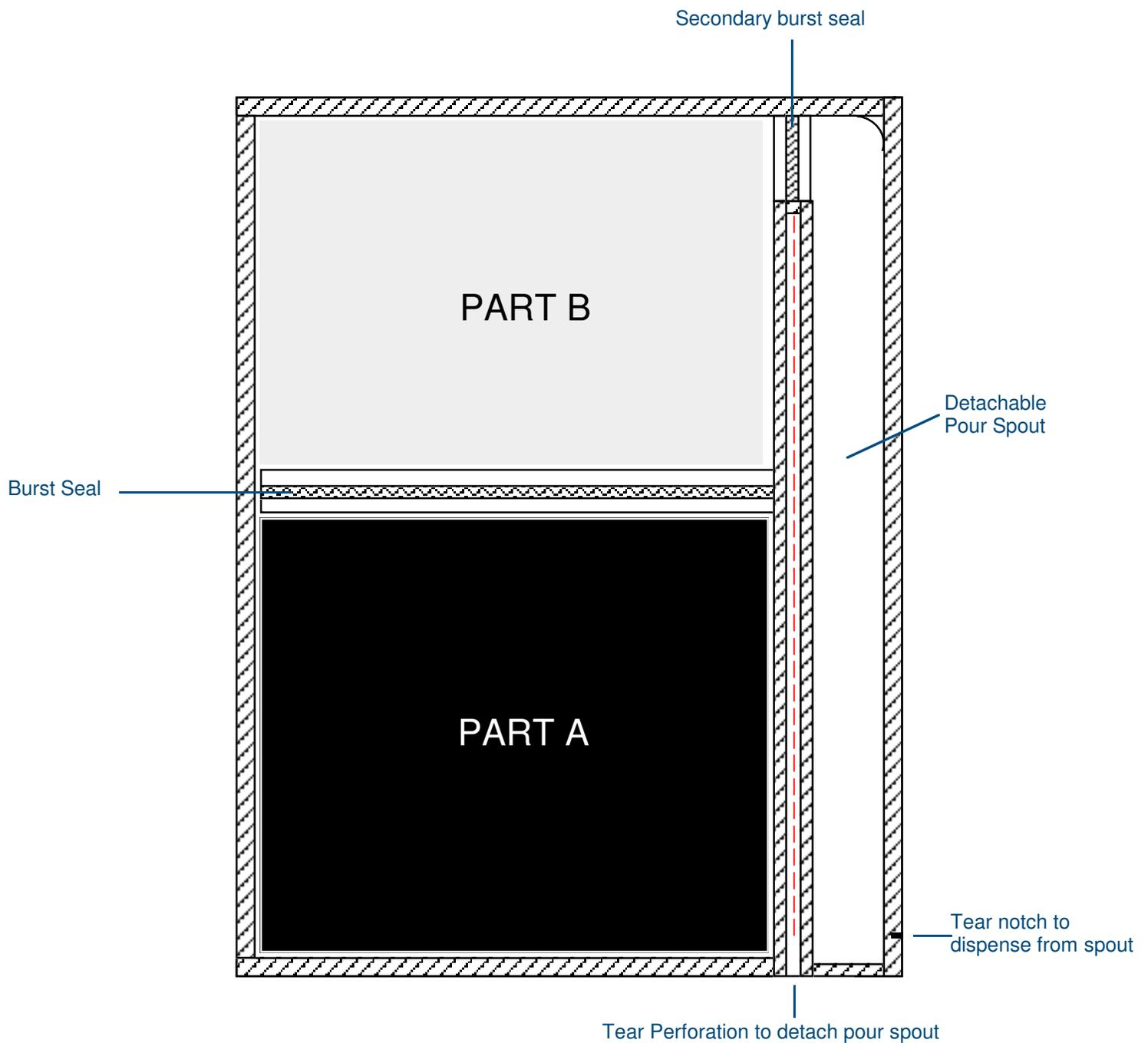
1. Mix the Part A and Part B like a conventional burst pouch.
